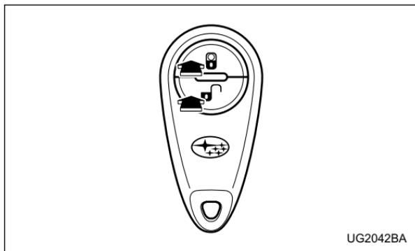
3. Press and release any button on the transmitter that you wish to program into the system. The horn will sound twice to indicate that the transmitter has been programmed.
