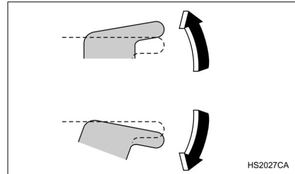
To open the passengers' windows, push the appropriate switch down and hold it until the window reaches the desired position.
