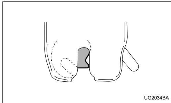
3. Move the release handle, from outside the vehicle, in the direction of the arrow to check if the latch is released.
