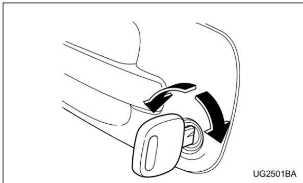
To lock the door from the outside with the key, turn the key toward the rear. To unlock the door, turn the key toward the front.
