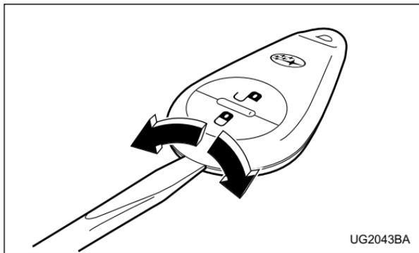
1. Open the transmitter case using a flat-head screwdriver.
