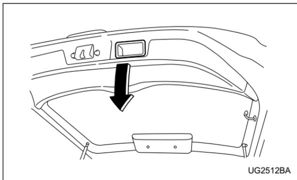
To close the rear gate, lower it slowly and push down firmly until the latch engages.
