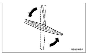
2. Turn the wiper blade assembly counterclockwise.
