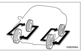
Tire wear varies from wheel to wheel. To maximize the life of each tire and ensure that the tires wear uniformly, it is best to rotate the tires every 7,500 miles (12,500 km). Rotating the tires involves switching the front and rear tires on the right hand side of the vehicle and similarly switching the front and rear tires on the left hand side of the vehicle. (Each tire must be kept on its original side of the vehicle.)
