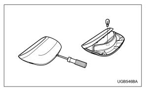
1. Remove the high mount stop light cover by prying the edge with a screwdriver.
