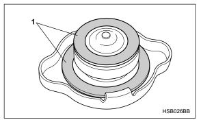
7. Put the radiator cap back on and tighten firmly. At this time, make sure that the rubber gasket in the radiator cap is correctly in place.
