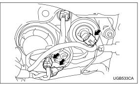
1. Remove two bolts and disconnect connectors.
