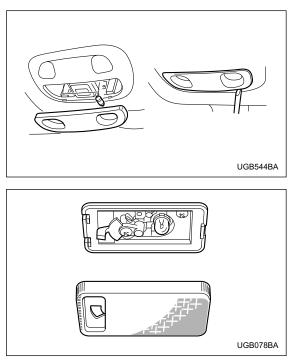
1. Remove the lens by prying the edge of the lens with
