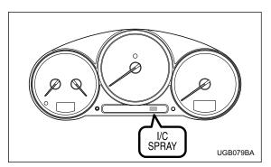
Add water to the intercooler water spray tank when the intercooler water spray warning light in the combination meter comes on. The warning light comes on when the water in the tank has decreased to approximately 0.4 liters (0.4 US qt, 0.4 Imp qt).
