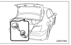
1. Remove the cover by squeezing its sides and pulling it.
