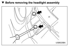
1. Loosen four clips at the top of the front bumper.
