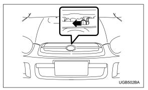
3. Release the secondary hood release located under the front grille by moving the lever toward the left.
