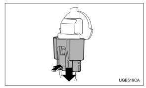
1. Disconnect the electrical connector from the bulb.
