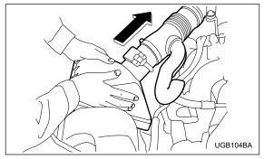
2. Push the air cleaner case cover in the direction of the arrow shown in the drawing.
