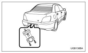
1. Remove the mounting screws using a Phillips screwdriver.
