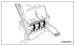
5. To install the air cleaner case cover, insert the three projections on the air cleaner case into the slits on the air cleaner case cover and then snap the two clamps on the air cleaner case cover.
