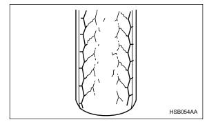
Ride comfort is poor. Also, the tire magnifies the effects of road-surface bumps and dips, possibly resulting in vehicle damage.
