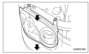
2. Pull the headlight assembly toward you and remove it from the vehicle.
