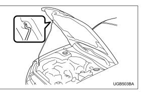
Lift up the hood, release the hood prop from its retainer and put the end of the hood prop into the slot in the hood.
