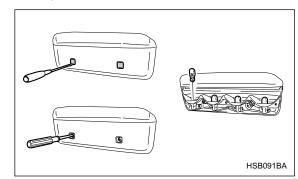
1. Remove the mounting screw covers by prying the edge with a screwdriver.
