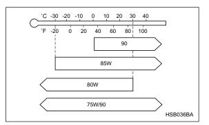
SAE viscosity No. and applicable temperature
