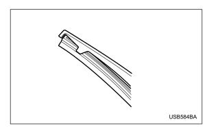
Securely retain both ends of the rubber with the stoppers on the plastic support ends. If the rubber is not retained properly, the wiper may scratch the rear window glass.
