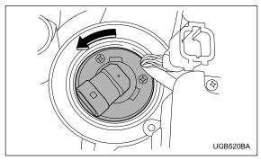
2. Remove the bulb from the headlight assembly by turning it counterclockwise.
