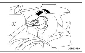
1. Remove the bulb socket from the headlight assembly by turning it counterclockwise.
