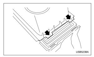
4. To install the air cleaner case cover, insert the two projections on the air cleaner case cover into the slits on the air cleaner case and then snap the two clamps on the air cleaner case cover.
