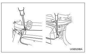
2. Remove the front grille. Use a screwdriver to detach the four clips at the top and the two hooks on each side. ▼ Removal of headlight assembly
