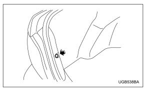
1. Remove the clip from the rear trunk trim with a screwdriver.
