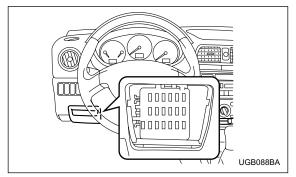
One is located under the instrument panel behind the coin tray on the driver's seat side.
