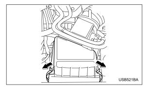
1. Unsnap the two clamps holding the air cleaner case cover.
