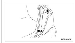
1. Using a Phillips screwdriver, remove the upper and lower screws that secure the side cover of the rear combination light assembly.
