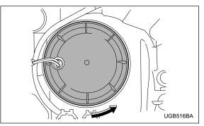
1. Remove the bulb cover, by turning it counterclock-wise.
