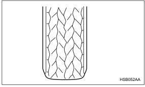
Roadholding is good, and steering is responsive. Rolling resistance is low, so fuel consumption is also lower. • Abnormally low tire pressure (tread worn at shoulders)
